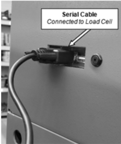
Figure 4–3. Serial Cable Connected to the Load Cell & USB/Serial Interface
