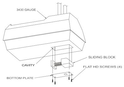
Figure 14. Cleaning the Tungsten Sliding Block
