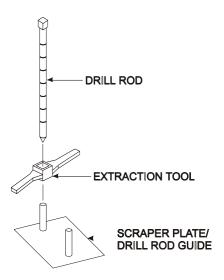
Figure 9. Drill Rod Positioning
