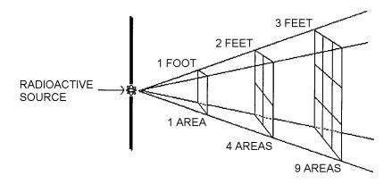
Figure 13. Effect of Distance on Exposure
