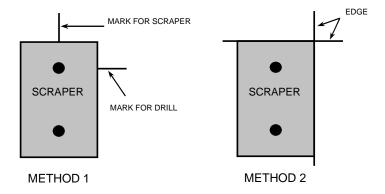
Figure 10. Marking the Test Area
