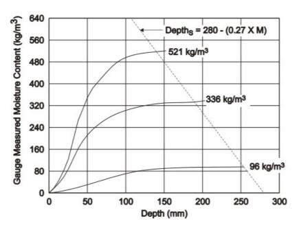
Figure 5. Effect of Moisture on Depth of Measurement
