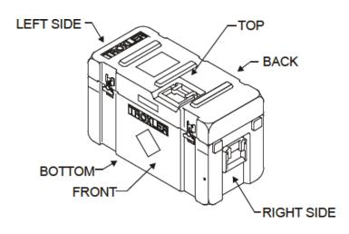
Figure 15. Model 3430 Gauge and Transport Case
