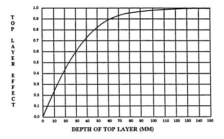
Figure 4. Backscatter Surface Density Effects
