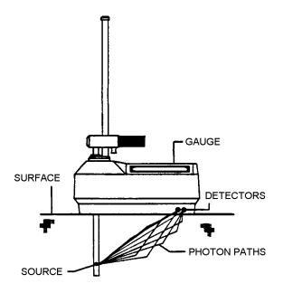
Figure 2. Direct Transmission Geometry
