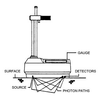
Figure 3. Backscatter Geometry
